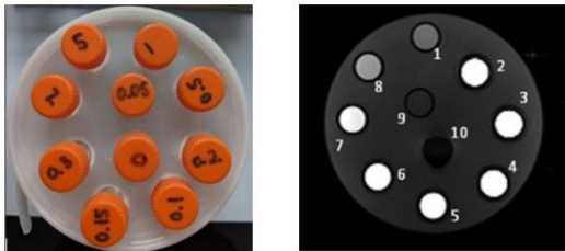
Figure 1 a) Plan view of the contrast phantom b) T1W MRI image of the contrast phantom
